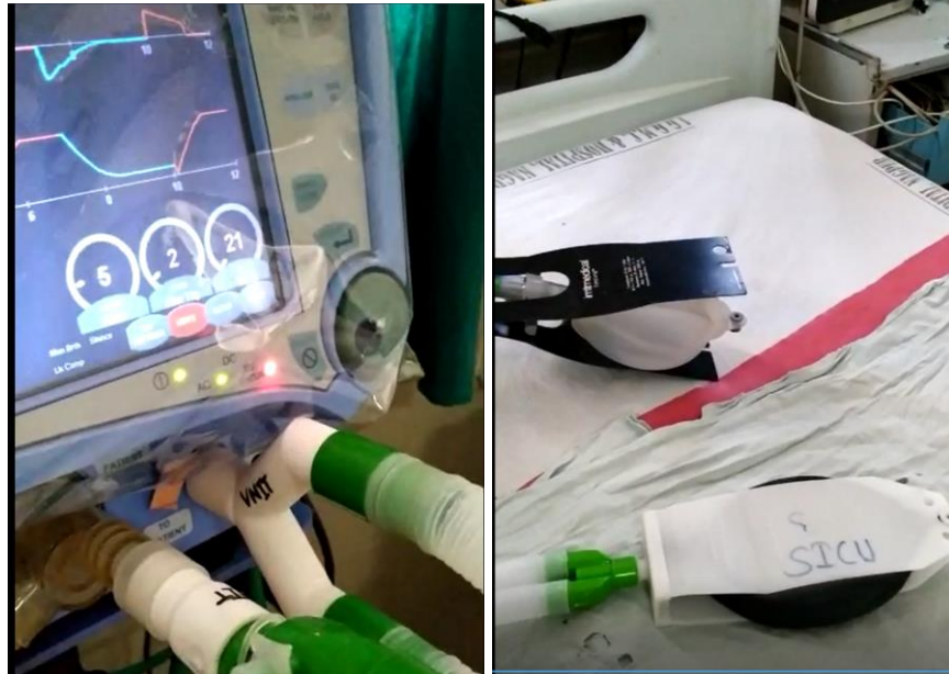
Splitters and restrictors developed by VNIT, during testing at IGGMC, Nagpur
