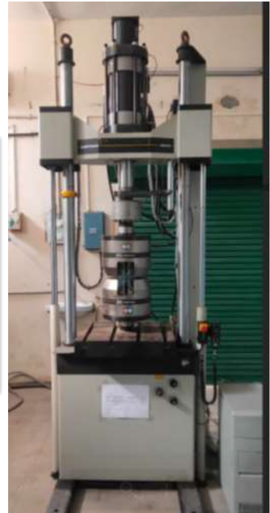
250 kN servo hydraulic Universal testing machine with high temperature attachment
