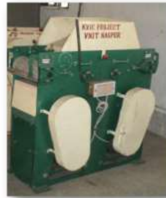
Modified Double Roller Gin
